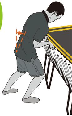
**5 Outside Person:** Push forward, rocking from your heels to the balls of your feet, using the weight of your body to push the white mat rod over the back edge of the mat rod holder. Keep the mat edge horizontal with your other hand.
