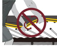
**10 Outside Person:** Do not twist or rotate the mat to remove a rod from a mat rod holder. This could cause serious injury or damage the trampoline.
